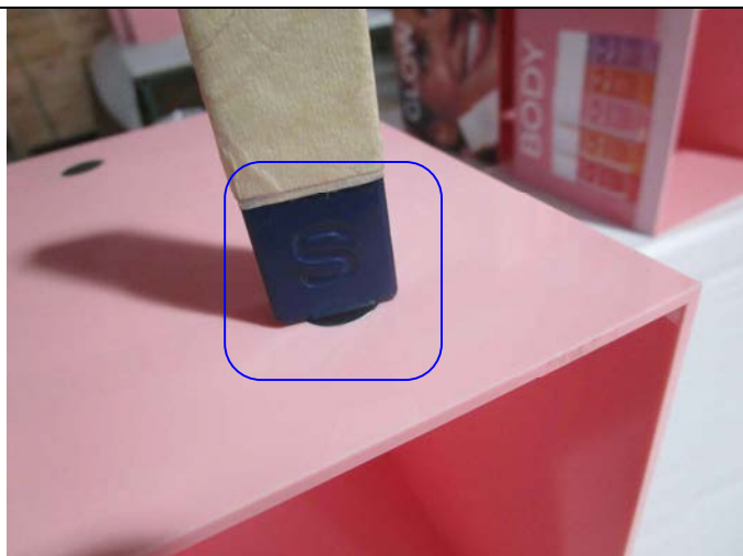
Magnet polarity installation is wrong
